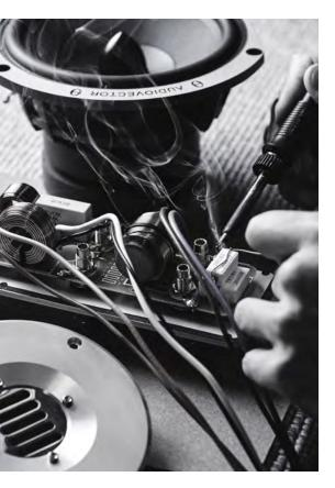
We engineer our own drivers, so they have the roll-off we want to be able to use smooth filtering, thus presenting a very easy load to the amplifier. We take pride in having high efficiency and careful mechanical decoupling. We use broad band damping material inside. Meticulously water-cut and exactly positioned. This is much better than random filling damping and is one of the criteria for accurate production.
